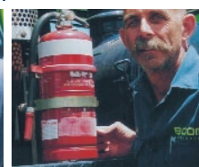
An essential item, a pressurised, dry powder, fire extinguisher unit. Usable on electrical fires.
