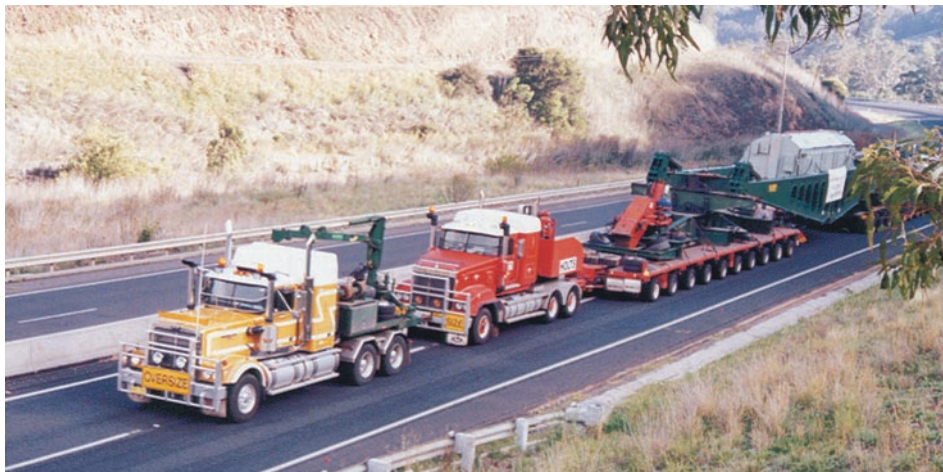
Two prime movers, each 550hp, hauling a 40 wheel float, load capacity 200 tonne.
